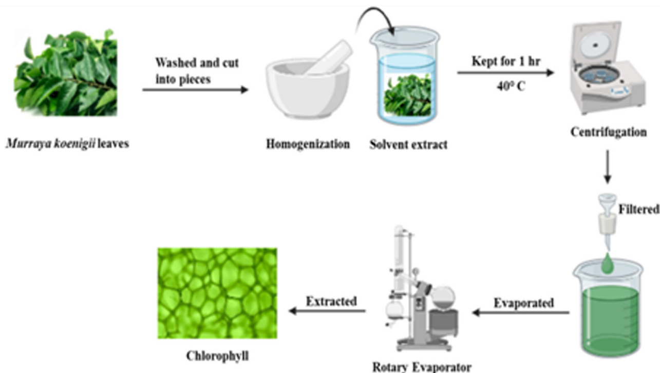
Figure 1: Schematic illustration of chlorophyll extraction process.
